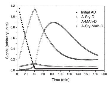
**Figure 4.**Relative concentrations of relevant species as a function of time determined via *in situ*<sup>1</sup>H-NMR spectroscopy during the CiPDB-mediated copolymerization of styrene and maleic anhydride at 70 °C. [STY]:[MAh]:[CiPDB]: [AIBN] = 4.1:3.8:1:0.20 [mol]. [12]
