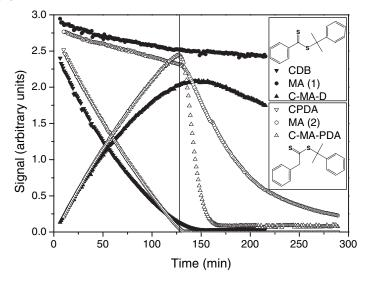
Figure 3. Relative concentrations of relevant species as a function of time determined via in situ<sup>1</sup>H-NMR spectroscopy during the polymerization of methyl acylate mediated by CDB and by CPDA [MA]<sub>o</sub>/[RAFT-agent]<sub>o</sub> = 7.5 at  $70^{\circ}$ C. [10]
