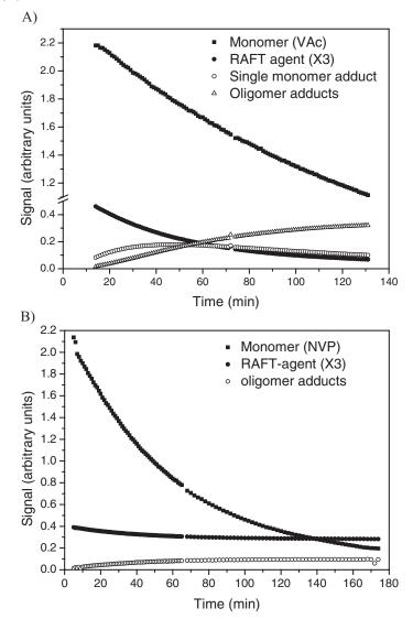
**Figure 7.** A and 7B. Relative concentrations of relevant species as a function of time determined via *in situ*<sup>1</sup>H-NMR spectroscopy during the *tert*-butyl ethyl xanthate (X3)-mediated polymerization of vinyl acetate (A) and of N-vinyl pyrrolidone (B) at 70 °C in  $C_6D_6$ , [Monomer] $_0$ /[Xanthate] $_0 = 5$ .[13]
