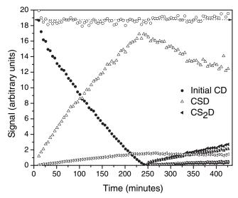
Figure 2. Relative concentrations of relevant species as a function of time determined via in  $situ^1H$ -NMR spectroscopy during the CDB-mediated polymerization of styrene at 70 °C, where C=cumyl fragment, S=styrene, D=dithiobenzoate. The non-assigned symbols are CiP-initiated chains as indicated in the CiPDB study (see Figure 1). [STY]:[CDB]:[AIBN] = 6.7:1:0.2 [mol]. [6]
