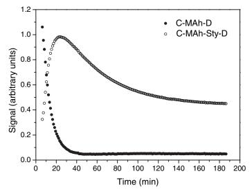
**Figure 5.** Relative concentrations of relevant species as a function of time determined via *in situ*<sup>1</sup>H-NMR spectroscopy during the CDB-mediated copolymerization of styrene and maleic anhydride at 70 °C. [STY]:[MAh]: [CDB]:[AIBN] = 3.6:3.6:1:0.2 [mol].<sup>[12]</sup>
