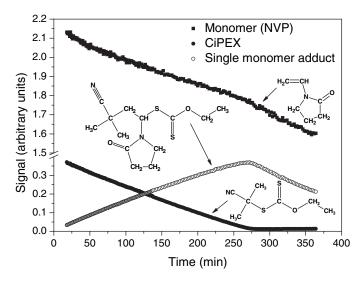
Figure 6. Relative concentrations of relevant species as a function of time determined via in  $situ^1H$ -NMR spectroscopy during the CiPEX-mediated polymerization of N-vinyl pyrrolidone at  $70\,^{\circ}C$  in  $C_6D_6$ , [Monomer]<sub>o</sub>/[Xanthate]<sub>o</sub> = 5.<sup>[13]</sup>
