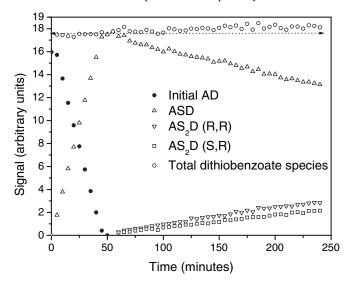
**Figure 1.** Relative concentrations of relevant species as a function of time determined via *in situ*<sup>1</sup>H-NMR spectroscopy during the CiPDB-mediated polymerization of styrene at 70 °C, where A = CiP fragment, S = styrene, D = dithiobenzoate. [STY]:[CiPDB]:[AIBN] = 5:1:0.1 [mol].<sup>[2]</sup>
